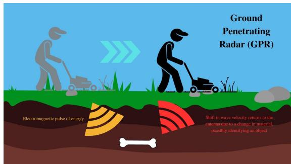
Professionals must be very careful to create their grid before using GPR. They also need a relatively flat, clear surface. The equipment must be used in straight, evenly spaced lines to make the best individual transects to be used later.
